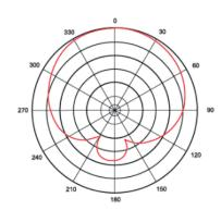
Directivity: Uni-directional Output connections: XLR (3-pin) Frequency Response: 50Hz - 15KHz
